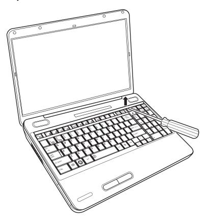
Figure 4.8 Removing the keyboard cover
