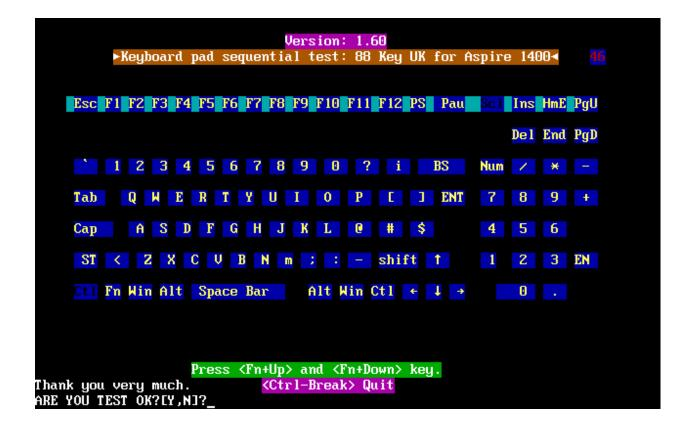
**NOTE:** The "Fn" key cannot be tested in the keyboard test. To determine whether the "Fn" key is working correctly, press "Fn+F6" or "Fn+F7" keys to check if LCD display brightness change gradually.
