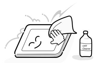
4. If water or other liquid is left on the panel's surface for a long period, it can change the screen's tint or stain it. Be sure to quickly wipe off any liquid.
